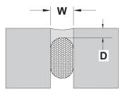
EXPANSION JOINTS - The minimum width and depth of any sealant application should be 1/4 in. by 1/4 in. (6mm by 6mm). The depth (D) of sealant may be equal to the width (W) of joints that are less than 1/2 in. wide. For joints ranging from 1/2 in. to 1 in. (13mm to 25mm) wide, the sealant depth should be approximately one-half of the joint width.
