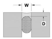
EXPANSION JOINTS - The minimum width and depth of any sealant application should be 1/4" by 1/4" (6mm by 6mm).
