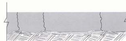
Uneven Grade Can Cause Cracking
