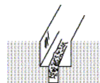
Close-up of crack before filling
