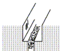
Close-up of crack before filling
