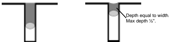
WRONG: Joint too deep. Poor shape for movement. RIGHT: Good width to depth ratio. Concave surface.
